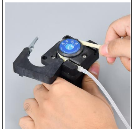
Step 3 Install the pump hose, and keep fittings on the two ends of the hose stuck to the pump head
